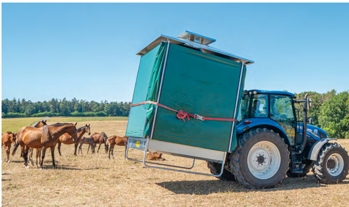
Transportation via 3-point linkage, when empty at max. 10 km/h, with down folded roof areas
