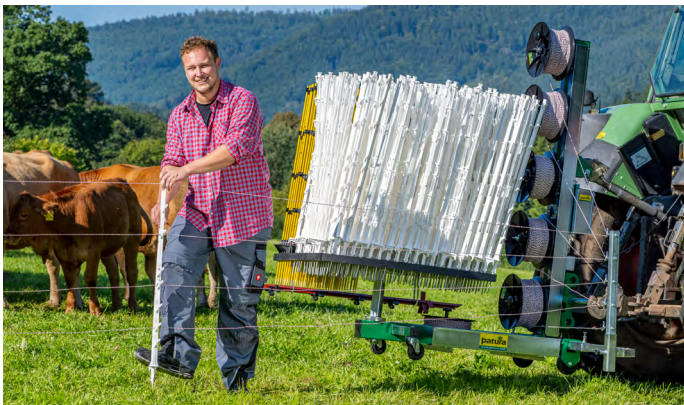
Exchangeable magazine for up to 400 posts
