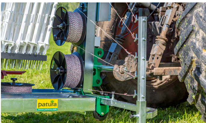
Up to 5 polywires and polytapes can be wound up or down in one run
