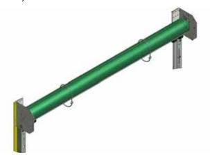
Figure 9, Tie Up Roller Assembly
